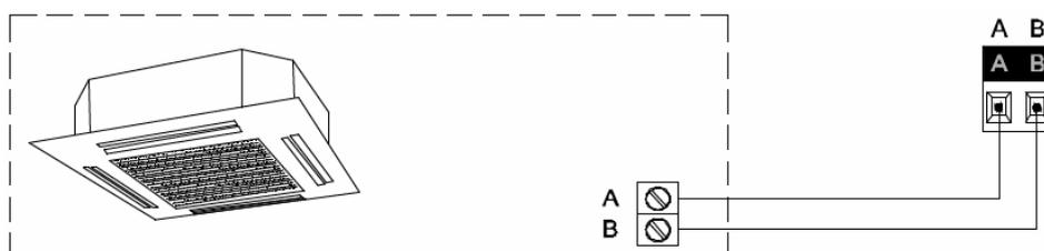
Figure 2. Connecting KLIC-TS to the A/C unit.
